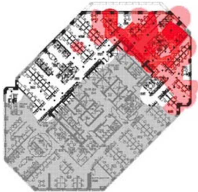
Figure 2 An example floor plan overlaid with a Wireless LAN signal coverage analysis. Areas with coverage can be seen in red.
