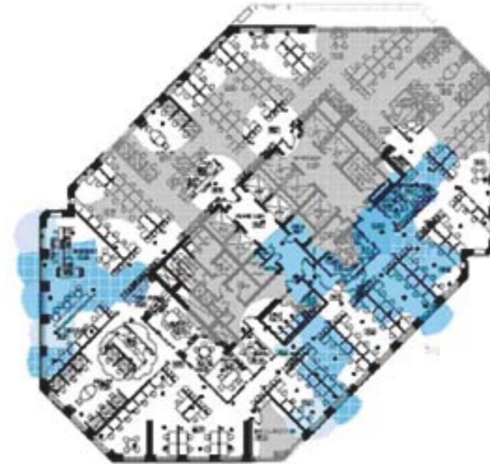
Figure 3 An example floor plan overlaid with a Wireless LAN interference analysis. Areas with interference can be seen in blue.
