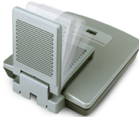
Figure 4 The design of the 802.11a radio module features an integrated omni directional and patch antenna.
