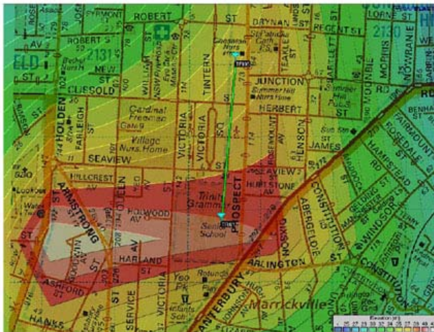
Figure 2 – Topographical view produced during a Path Loss Analysis
