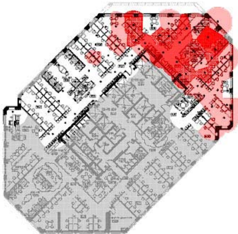
Figure 5 – An example floor plan overlaid with our WLAN signal coverage analysis
