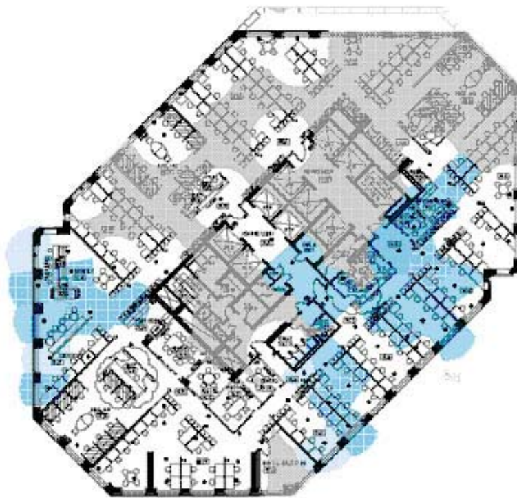
Figure 6 – An example floor plan overlaid with our WLAN interference analysis.
